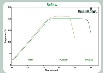
This profile is designed for use with **Durafuse® LT** (Indium10.8HF). This can be used as a general guideline in establishing a reflow profile for **Durafuse® LT** Solder Paste. Deviations from these recommendations are acceptable, and may be necessary, based on specific process requirements.
