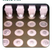
Indium Corporation uses several of its own tests, based on IPC workmanship standards, for determining hole fill. Depending on the design criteria for the flux, Indium Corporation uses holes of varying sizes and circuit board finishes. However, we always look for 100% hole fill, even
