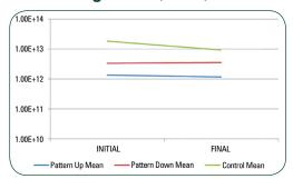
The electromigration test is performed to IPC-TM-650 method 2.6.14.1 with boards prepared using IPC-TM-650 method 2.6.3.3. The test conditions for this test are 496 hours at 65°C  $\pm$ 2°C and 88.5%  $\pm$ 3.5% RH. To pass this test, there should be no visible corrosion and no dendritic growth that decreases line spacing by more than 20%. In addition, the insulation resistance
