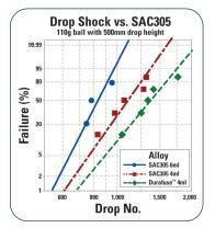
Durafuse™ LT samples in the chart (left) experienced a peak reflow temperature of 210°C and demonstrated drop shock resilience similar to that of SAC305.
