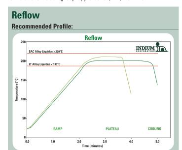
This profile is designed for use with **Durafuse™ LT** (Indium10.8HF). This can be used as a general guideline in establishing a reflow profile for **Durafuse™ LT** Solder Paste. Deviations from these recommendations are acceptable, and may be necessary, based on specific process requirements.
