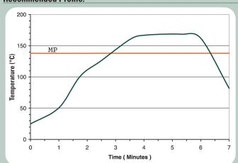
This profile is designed for use with Indalloy<sup>®</sup>281 and can serve as a general guideline in establishing a reflow profile for use with other alloys. Adjustments to this profile may be necessary based on specific process requirements.
