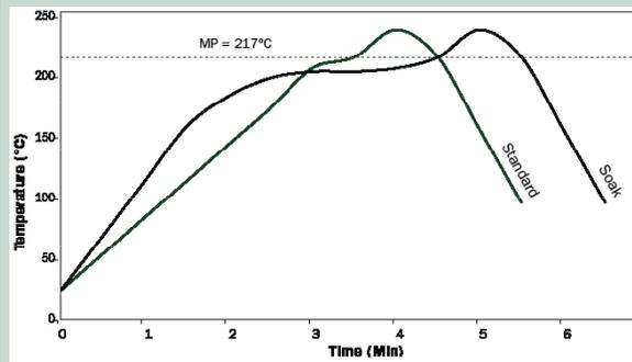
The stated profile recommendations apply to most Pb-free alloys in the SnAgCu (SAC) alloy system, including SAC 305 (96.5Sn/3.0Ag/0.5Cu). This can be used as a general guideline in establishing a reflow profile when using Indium8.9HFA solder paste. Deviations from these recommendations are acceptable, and may be necessary, based on specific process requirements, including board size, thickness & density.
